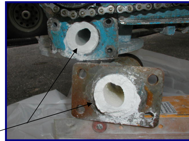
Calcium carbonate scale generated at MLC's Ste. Genevieve R&D facility
